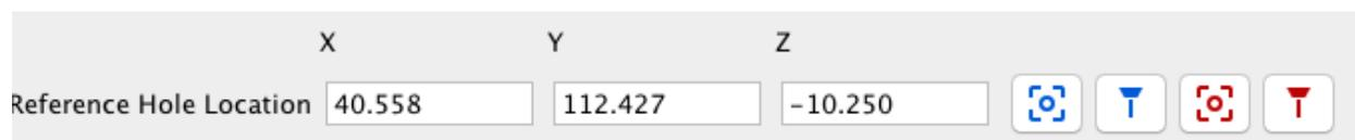
The buttons control the fields and respond to the values in them. You'll also see the buttons used individually where applicable, like in the Job tab. Here the buttons are used in context with the selected board to capture the board location or move to it.
